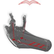
Test your speed system for the correct length of cord on the ground first (simulating flying position), with your harness and risers, before flying with it! The full range is reached when the 2 pulleys join together.
